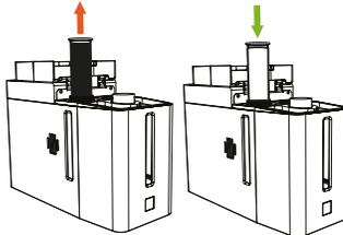
**Step 5:** Remove the saturated desiccant capsule and replace with a fresh capsule.
