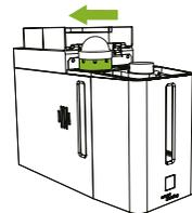
**Step 6:** Replace the cap and place the tool on top, tighten with the tool by turning it clockwise.
