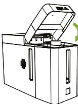
**Step 7:** Close the top panel. The de-ionizer cartridge will need to be changed after 12 months.
