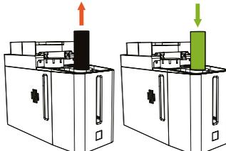
**Step 5:** Remove the de-ionizer cartridge and replace with a fresh cartridge.
