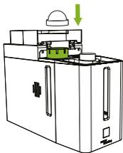
**Step 4:** Loosen and remove the cap of the desiccant dryer by placing the tool onto the cap and turning counter-clockwise.
