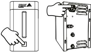
**Step 1:** Press and hold the power button for 5 seconds to shutdown and depressurize. Now turn off the main power switch at the back of the unit.
