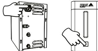
**Step 8:** Power up the generator using the main power switch on the rear of the unit. Once diagnostics are complete, the LEDs will be solid green and the generator will be ready to deliver gas to the application. Press the front button to supply gas to the application.
