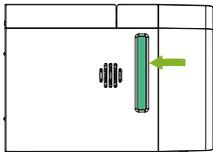
**Step 1:** Check Silica gel colour via the window on the left-hand side panel of the generator (if blue/green it needs to be replaced).
