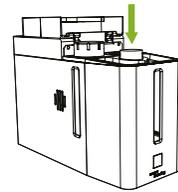
**Step 3:** The de-ionizer cartridge is located in the water tank and can be accessed by opening the top panel.
