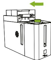
**Step 6:** Fix replacement de-ionizer cartridge in place by turning clockwise.
