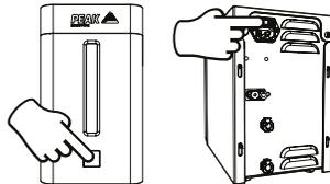
**Step 2:** Press and hold the power button for 5 seconds to shutdown and depressurize. Now turn off the main power switch at the back of the unit.
