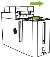
**Step 4:** The de-ionizer cartridge can be removed by turning the cartridge counter-clockwise.
