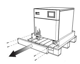
Remove the four screws shown, these will be marked in red and remove the front bar.
