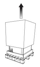
Remove cardboard lid, protective foam packaging and cardboard sleeve. Remove the plastic covering the generator.
