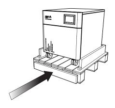
**Place** the front bar against the front of the pallet. Failure to complete this step can cause damage to the generator.
