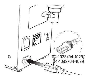
Select the appropriate **mains cable** from the fittings kit and plug the **IEC 60320/C19** cable into the **mains input** at the side of the generator.
