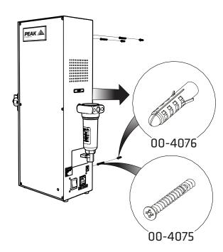
With the holes drilled in your desired location, fit the  $3 \times 10.8$  Wall Plug 00-4076 and  $3 \times 10.8$  Screw 00-4075 to the wall and mount your generator onto them.
