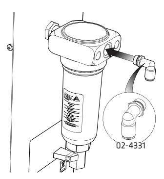
Select the 1/4" - 6mm Push Fit Elbow Fitting 02-4331 and attach it to the filter outlet on the right side of the generator. It is recommended that PTFE tape is applied to the threads to ensure a leak-tight fit.
