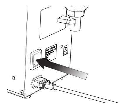
Swith the generator **ON**, using the **switch at the side** of the generator.
