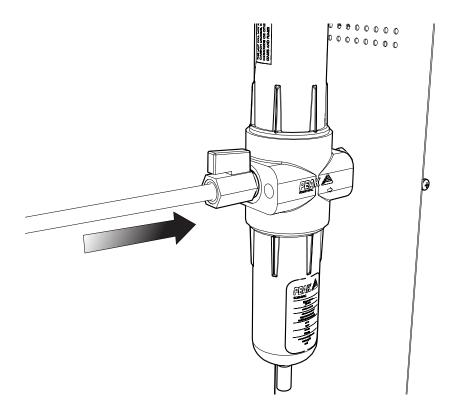
Attach your house air supply to the **BA filter** at the **left side** of the generator. Ensure the valve on the filter is at the **open** position.
