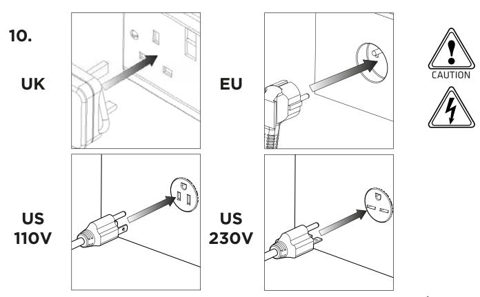
Plug the mains cable into the corresponding **110VAC 60Hz OR 230VAC 50/60Hz** single phase power supply.
