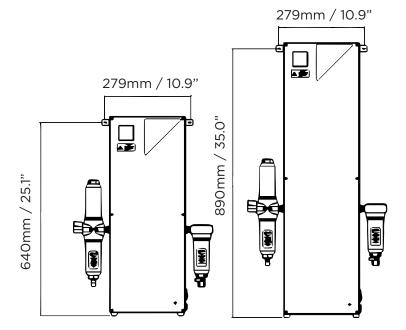
Finally, using the dimensions provided, fix the wall plugs to the wall, ensuring that the wall plugs provided are suitable for the type of wall in question. Secure the generator to the wall with the screws from the fittings kit.
