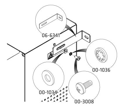
If the generator is not wall mounted using the key slots in the rear face, it must be fixed to the wall using the brackets provided for safety reasons.
