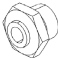
x2 1/4" BSPP x 6mm Push Fitting 3304226
