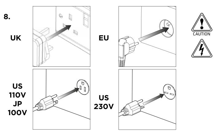
Plug the mains cable into the corresponding 100/110/230VAC 50/60Hz single phase power supply.
