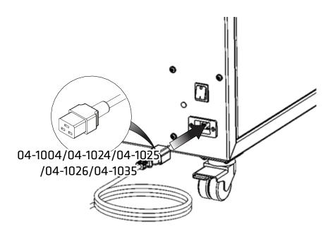
Select the appropriate mains cable from the fittings kit and plug the IEC 60320/C19 cable into the mains input at the rear of the generator.
