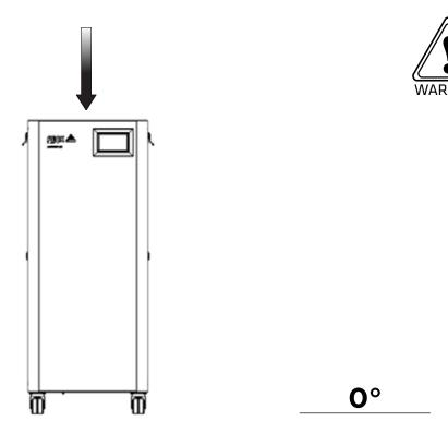
Unpack the generator from the shipping crate and **position on a flat surface**, in desired area.
