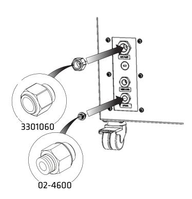
Select the 16mm Push Fit Fitting 3301060 from the fittings kit and attach to the Air Inlet port at the rear of the generator.
