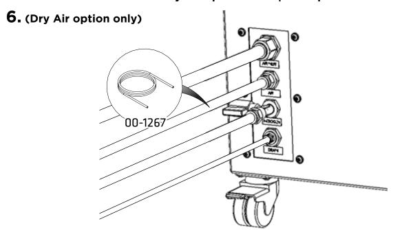
Attach 3m of 12mm PE tubing 00-1267 from the fittings kit to the fitting on the Dry Air output of the generator. Connect the other end to the Air inlet of your instrument.
