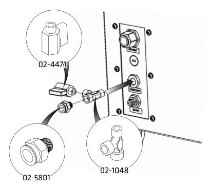
Select the Tee Fitting 02-1048 and attach this to the Nitrogen port.
