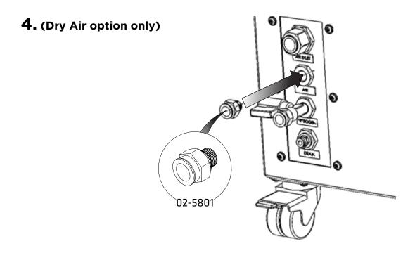
If the generator is fitted with the optional **Dry Air output**, select the **12mm Push-Fit Fitting 02-5801** from the fittings kit and attach it to the 'Air' port on the rear of the generator.
