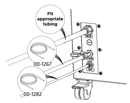
Connect the 6mm PE Tubing 00-1282 to the 1/4"- 6mm Push Fit Fitting 02-4600.
