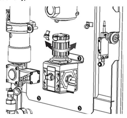
Set the desired Air output pressure using the internal pressure regulator located near the rear of the generator. View the external outlet pressure reading on the HMI when setting the pressure. Replace the side panel after the regulator has been set.
