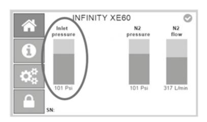
The inlet pressure graph on the external HMI of the generator will gradually increase from OPsi to the delivered inlet pressure as the system pressurises
