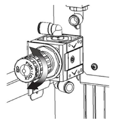
Remove the side panel, and set the desired Nitrogen output pressure using the internal pressure regulator located near the front of the generator. View the external outlet pressure reading on the HMI when setting the pressure.
