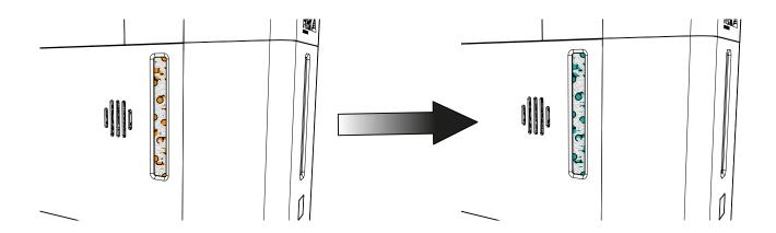
1. To replace the capsule, **depressurise the generator and disconnect power.** Lift the hinged lid back, then unscrew and remove the capsule cap anticlockwise, using the dryer cap removal tool.
