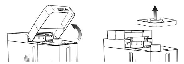
2. Fill the water tank from your lab's supply of DI water, and ensure the tank cover is replaced, afterwards.
