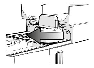
2. Next withdraw the inner tube and dispose as per your company's hazardous waste disposal policy and MSDS guidelines. The new capsule may now be inserted into the outer collar.
