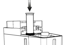
3. The cap can then be replaced again using the dryer cap removal tool, ensuring not to over-tighten the cap and the hinged lid can be closed.
