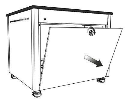
Remove the front panel, ensuring that the fan power is disconnected.
