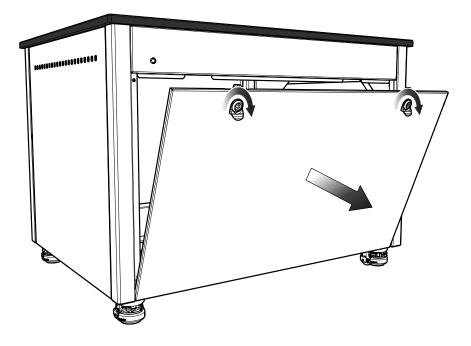
Remove the front panel, ensuring that the fan power is disconnected.
