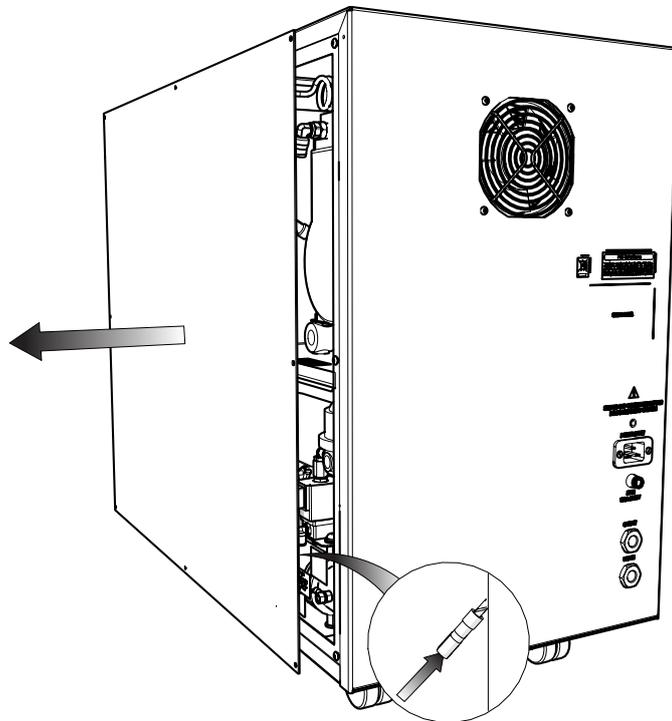
The side panel can now be **removed**, an **earth lead** is connected to the inside of the panel. This can be **disconnected** by pulling it off the spade connector on the panel.
