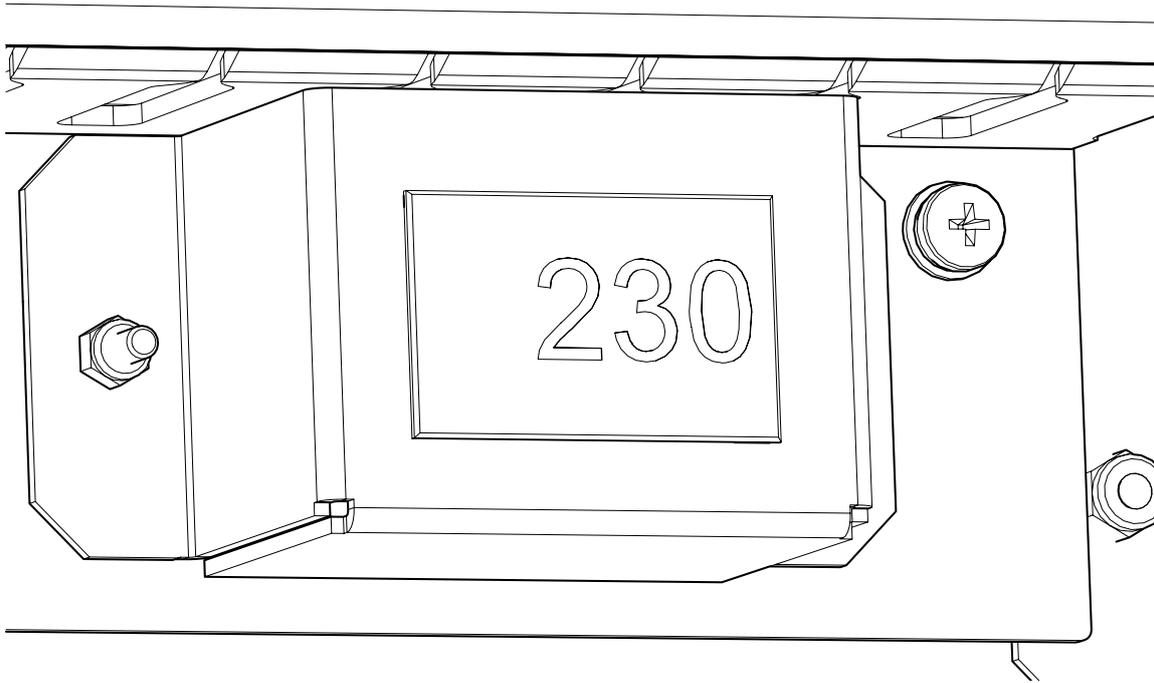
Check the Generators **internal voltmeter**. This will measure and display the mains voltage that is being supplied to the generator. Note the displayed voltage. If the voltage is 219V or less, we would highly recommend fitting a transformer. This can be ordered directly from Peak. **06-3200 Dual Tap Transformer 200-230V**
