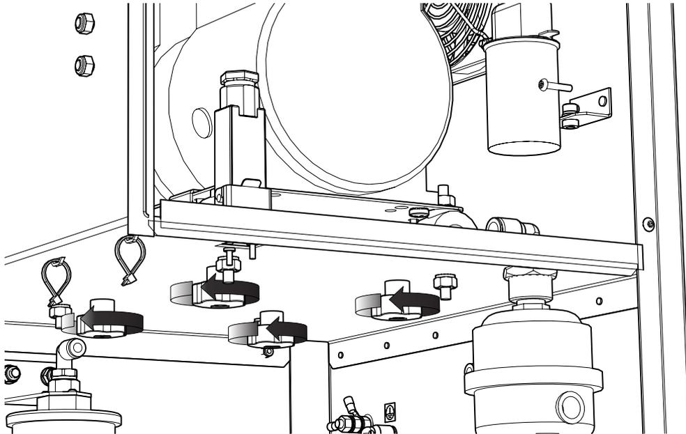
**Remove the four thumb-screws and shake-proof washers** from the underside of the compressor compartment. Then **lift each transit bracket up** until the locating pin and threaded stud are clear of the mounting plate and the compartment floor.
