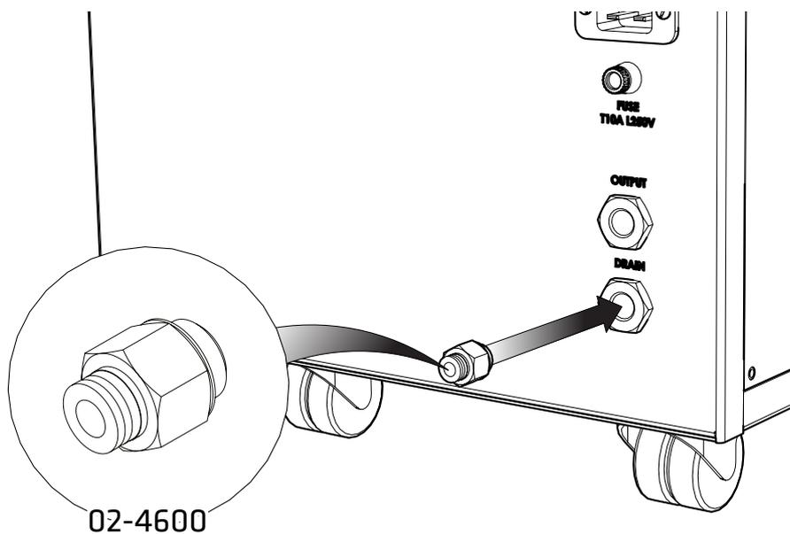
Select the  $\frac{1}{4}$ "- **6mm Push Fit Fitting 02-4600** and attach to the Drain port at the rear of the generator.
