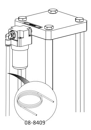
The outlet of the unit is fitted with a particulate filter and a 6mm push-fit elbow. Connect the 6mm PE tubing provided here and connect to your application.
