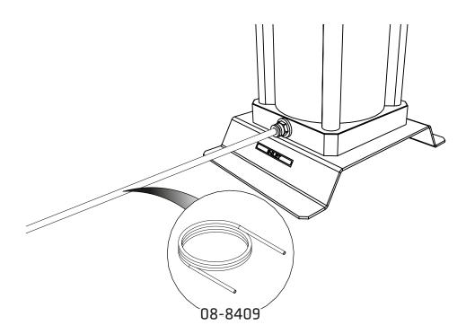
The unit is fitted with a 6mm push-fit connection at the inlet. Connect the 6mm PE tubing provided here and connect the other end to your gas supply.
