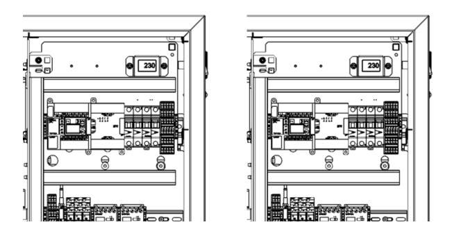
For the N118LA, the voltmeter is located on the control panel.
