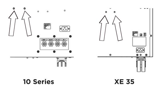
Find the location on the generator where the transformer is fitted. This can be done by looking for the M6 clinch nut threads, usually on the back on the generator.
