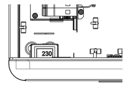
The voltmeter should now read above 220V. If it is still below 220V and you have not fitted the '208V tap', disconnect the transformer and return to step 14.
