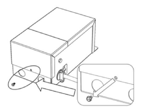
Place the transformer on its back and remove the cover retaining screw using either a flat blade screwdriver or ¼" spanner. The cover can then be removed.
