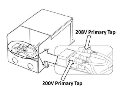
The 'Primary Taps' are now exposed. These are clearly labelled '200V' and '208V'. To change the tap simply pull the connector labelled '200V' off the spade terminal and push the connector labelled '208V' fully on to the terminal. The '200V' tap wire removed can be safely left loose in the compartment.
