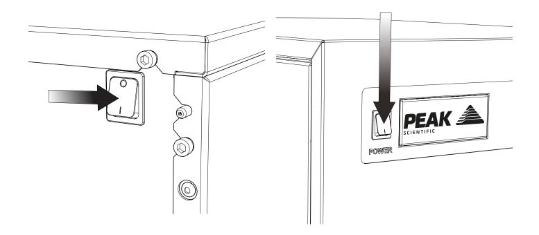
Ensure that the generator to which the transformer is to be fitted is switched OFF by the green rocker switch, located at the front (10 Series, NM32LA, N118LA) or the rear (QSD, SMZ, XE35) of the generator.
