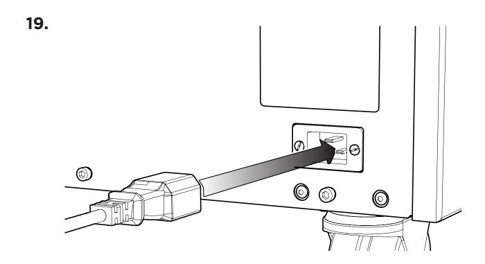
Plug the mains cable from the transformer, labelled 'TO GENERATOR' into the mains socket on the rear of the generator.
