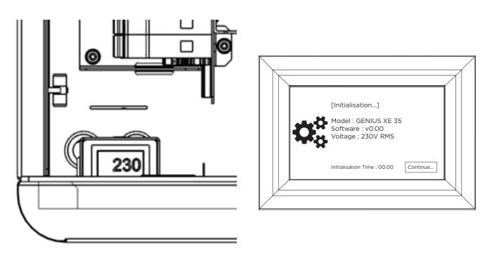
For Genius XE35 the volt meter is located at the top of the genetrator, and is mounted next to the fascia. For Genius XE 35 built pre November 2021 the voltage can be read from the HMI.
