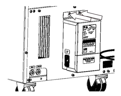
The mounting screws provided can be screwed into the holes on the rear of the generator. Leave approximately 5mm protruding. The transformer can then be hung on the protruding screws. Once located correctly the screws can be fully secured.
