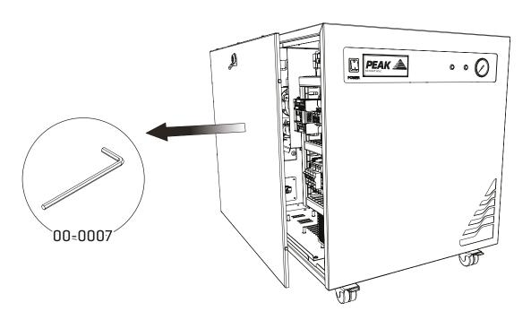
Use the 8mm Hex Key 00-0007 to turn the lock anti-clockwise, and remove the side door.
