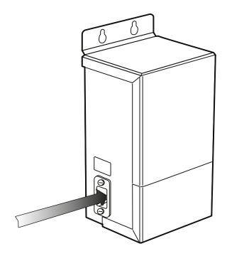
Plug the original generator mains cable into the mains inlet socket on the transformer, labelled 'MAINS INPUT'.
