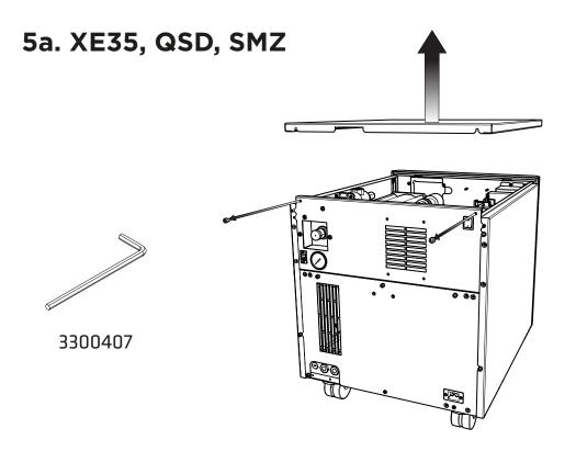
Use the **4mm Hex Key 3300407** to loosen the **two cap screws** fixing the top plate to the rear of the generator, then **tilt up and slide backwards to release the top plate** from the generator.
