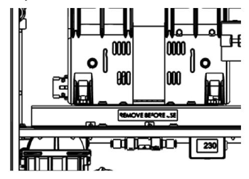
For 10 Series and NM32LA, the voltmeter is fitted under the compressor compartment.
