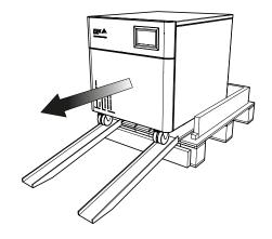
Release the brakes and **carefully manoeuvre Generator** down the ramps and into final position.
