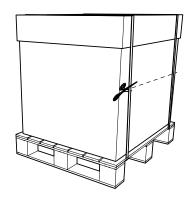
**Cut** the plastic strapping and **remove**.
