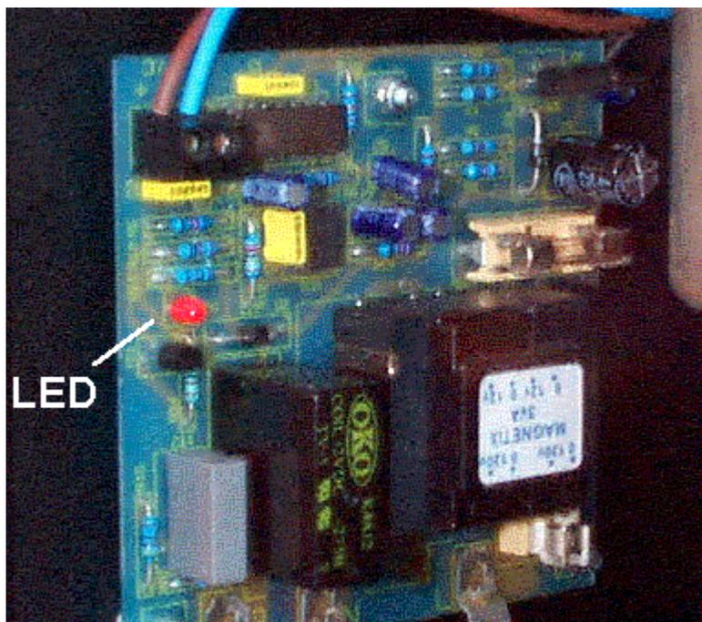
After a period of time (around 40 minutes) the Catalytic Chamber should have reached the required temperature. When this happens the relay on the Temperature Controller will “click” and the red LED will go out. The heater will then cycle on & off as required.
