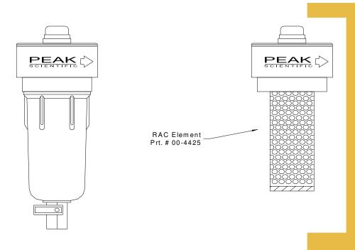
The filter housing is removed by un-screwing in a counter clockwise direction IMPORTANT!!! Ensure that the system is NOT under pressure before attempting to remove the bowl and that the air supply is shut-off.
