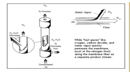
Air passes into the system via the *Breathing Air Filter*. This will prevent bulk moisture and harmful contaminants from reaching the Membrane. The clean air then passes into the Membranes where Oxygen, CO2 and Moisture are removed allowing High Purity Nitrogen to pass through. The Output Flow is regulated for pressure and then passed through an *Activated Carbon* Filter to ensure no carry-over of harmful contaminants
