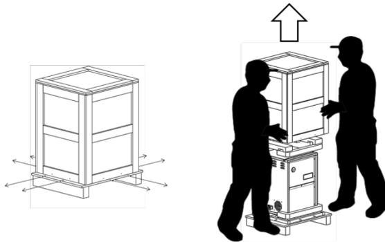
The generator can now be lifted out of the crate base and onto the floor. This should be done again with someone positioned at either side. There is a gap in the foam base for hand access; one hand should be positioned here underneath the generator and the other at the back supporting the weight. The generator should then be tilted back slightly and then up and out of the foam base and onto the floor.
