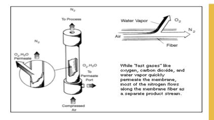
Air passes into the system via the *Breathing Air Filter*. This will prevent bulk moisture and harmful contaminants from reaching the Membrane. The clean air then passes into the Membranes where Oxygen, CO<sub>2</sub> and Moisture are removed allowing High Purity Nitrogen to pass through. The Output Flow is regulated for pressure and then passed through an *Activated Carbon* Filter to ensure no carry-over of harmful contaminants
