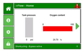
The Red warning triangle in the top right corner of the screen, indicates a fault condition is active on the system. Pressing the icon will take you to the Error page which will include a full description of the fault.
