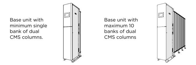
The front end cabinet, control system and valves are consistent across the entire range. To increase the outlet capacity, as you go up the range of generators, additional banks of CMS columns can be added. (Note: Mini models with 3-4 & Prime models with 5-10 banks require additional vent valves & silencers fitted to the rear of CMS column assembly).
