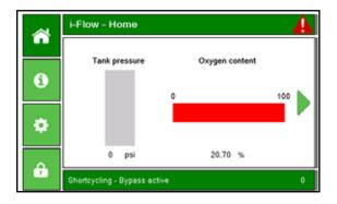
Initially, the generator should show 0 pressure in the tank, and nominal 20.7% ambient O2 content, at this point the system will be shortcycling, automatic bypass feature will be active, and the generator will be internally venting "bad" gas:
