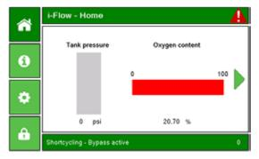
This is the Main Home page screen at first startup of the system. Error Icon in the top right of the screen is Normal, as pressure will be low and O2 content will be high. Touching the red triangle icon, will take you to the error page. In the bottom green bar the system status will be shown on the left side and the current cycle time on the right side.
