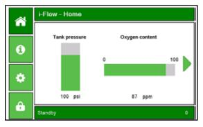
The system will continue to produce Gas until the Standby pressure is reached, at which point the generator will enter the "Standby" mode.
