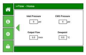
This is the second page of the home screen, showing the additional and optional sensor readings. This screen is accessed by the green arrow on the right hand side of the main Home Screen, to return press the green arrow on the left hand side of this screen.
