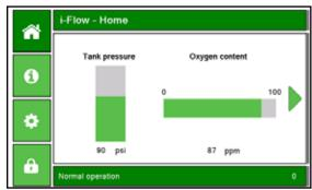
Once the desired tank pressure has been achieved, the system will automatically exit the "Shortcycle" mode and begin "Normal Operation".
