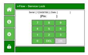
This is the Service Lock Screen - only trained and authorised engineers will have the ability to enter a PIN code and access generator settings and parameters. If the wrong PIN is entered too many times the screen will lock.
