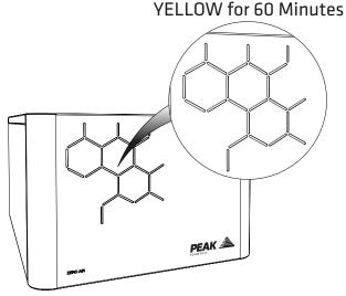
On completion of the start-up period, up to 60 minutes, the fascia will illuminate **GREEN** or **BLUE (70-\*\*\*\* Part Numbers Only)**. The generator is now ready to be used.
