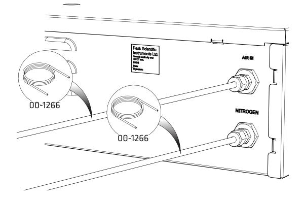
Connect the supplied 1/4" **Teflon Tubing** to the **AIR IN & NITROGEN** ports. Connect the other ends to the instruments gas inlets.
