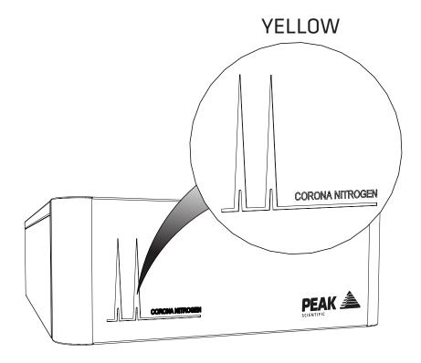
The  $\bf LEDs$  on the front of the generator should now illuminate  $\bf YELLOW$  as the unit starts up.
