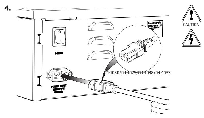
Select the appropriate mains cable from the fittings kit and plug the **IEC 60320/C13** cable into the mains input at the rear of the generator.
