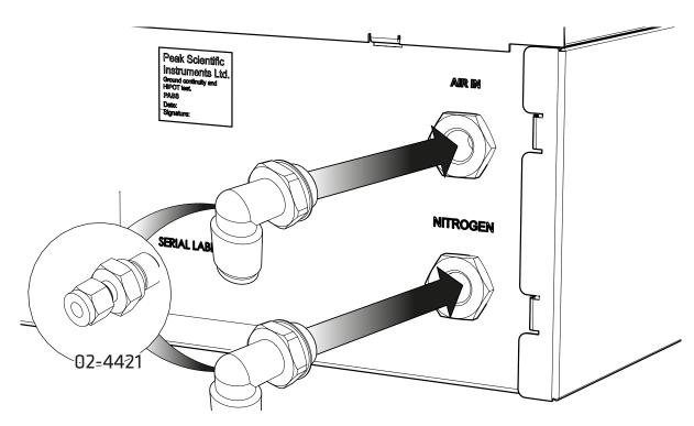
Select the  $\frac{1}{4}$ " x  $\frac{1}{4}$ " Compression Fittings and attach to the AIR IN and NITROGEN ports.
