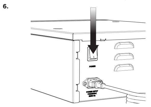
Press the **POWER** switch located at the rear of the generator.
