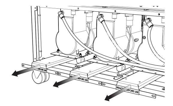
With the screws removed, **slide each transit bracket out** from underneath the compressor.
