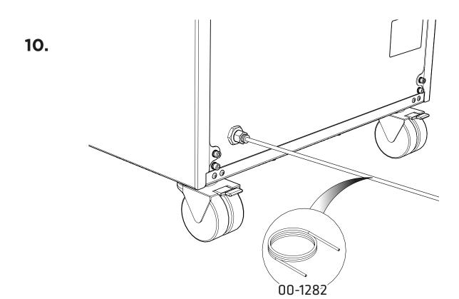
Connect the 6mm PE Tubing 00-1282 to the 1/4"- 6mm Push Fit Fitting 02-4600.
