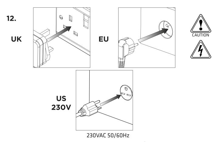
Plug the mains cable into the corresponding **230VAC 50/60Hz** single phase power supply.
