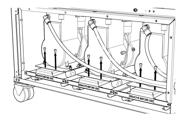
Remove the **2 x M5 cap screws** on each compressor base plate, using the **4mm Hex Key 3300407**.
