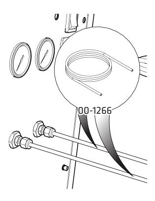
Attach the ¼" Teflon tubing 00-1266 to the fittings attached to the Nitrogen and Air ports and connect to the corresponding gas inlets of your instrument.
