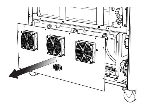
Remove the compressor fan panel.
