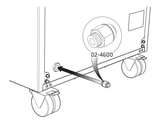
Select the ¼"- 6mm Push Fit Fitting 02-4600 and attach to the Drain port at the rear of the generator.
