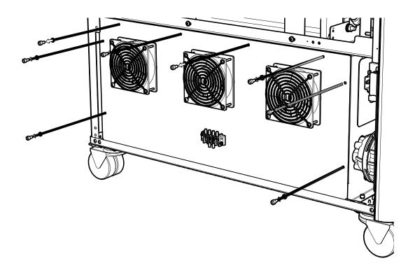
The **transit brackets** are located below the compressors inside the compressor compartment. Disconnect the fan power cables, then using the **4mm Hex Key 3300407**, remove **8 x M5 cap screws and washers** and keep in a safe place.
