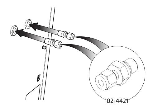
Select the 1/4" Compression Fittings 02-4421 and connect to the Nitrogen and Air ports.
