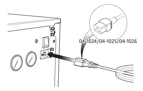
Select the appropriate **IEC 60320/C19** mains cable from the fittings kit and plug the cable into the mains input at the rear of the generator.
