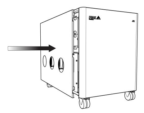
Replace the **6 x M5 pozi drive screws** and washers to secure the compressor trays. Replace the compressor fan panel, ensuring the fan power cables are reconnected and finally replace the left hand side panel.
