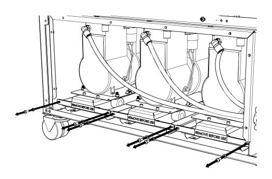
To **remove the transit brackets**, remove the **2 x M5 pozi drive screws and washers** on each compressor tray, using a pozi drive screwdriver (not supplied.)
