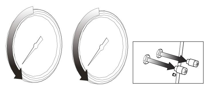
The purge is now complete. Once the pressure gauges at the rear of the generator read 0, the **silencer fittings can be removed** from the **Nitrogen** and **Air** ports.
