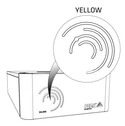
The **LEDs** on the front of the generator should now illuminate **YELLOW** until the unit reaches operating pressure.
