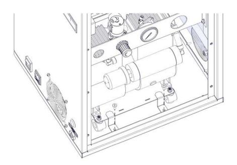
Now **locate the red transit bracket** attached to the compressor foot plate, and **remove the two screws** on the bracket.
