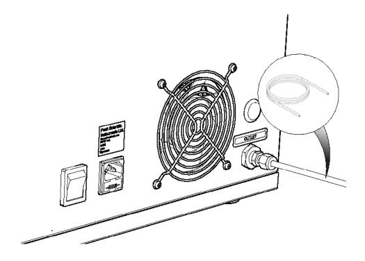
Attach suitable tubing to the generator's outlet. Either a 6mm,  $\frac{1}{4}$ " or  $\frac{1}{8}$ " diameter tubing will be suitable depending on your needs. If you are unsure please contact us.
