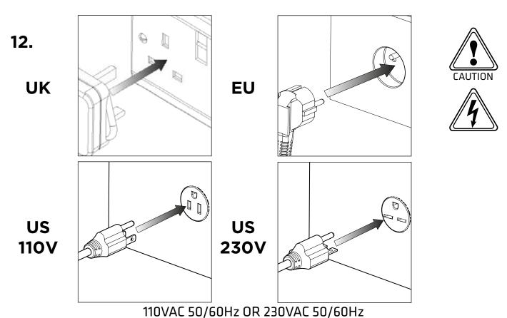
Plug the mains cable into the corresponding 110VAC 50/60Hz OR 230VAC 50/60Hz single phase power supply.
