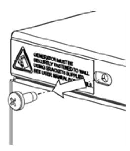
Remove the screw from the generator this should be repeated for the other side of the unit, and retain.
