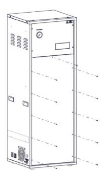
For NG 3000-5000(A) before the unit is used, the transit brackets must first be removed from the compressor.
