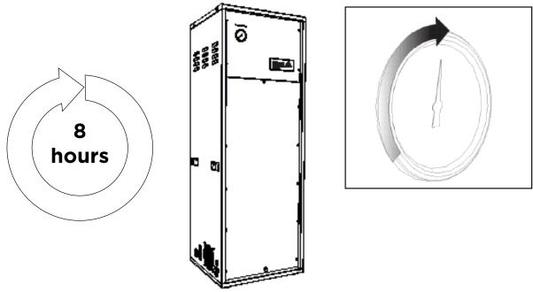
Leave the generator **switched on** for a period of **8 hours** to purge the system. The **pressure gauge** on the front panel will gradually increase to the factory set pressure.
