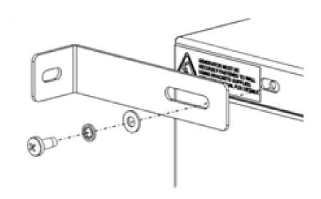
Next, **using the screw which was removed**, fit the **bracket and washers** provided to the generator. Again this should be repeated for the other side. The bracket is adjustable to accommodate varying kickboard widths.
