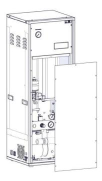
Then **remove the front panel** from the generator.
