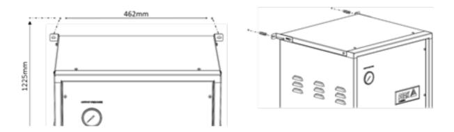
Finally, using the dimensions provided, **fix the wall plugs to the wall**, ensuring wall plug is suitable for the type of wall. If not, use the correct type. **Secure the generator to the wall** with the screws from the fittings kit.
