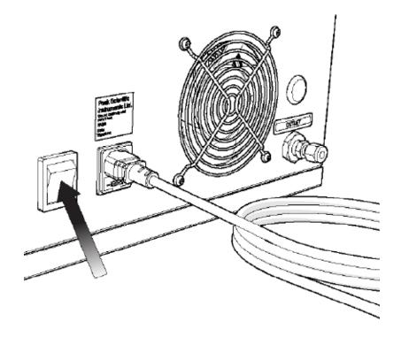
Switch the generator power **ON** using the switch on the side of the unit.
