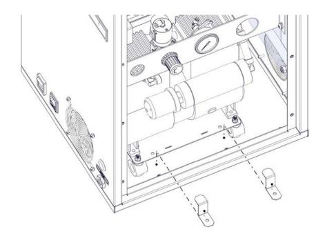
Next **remove the transit bracket** by first lifting up and then out of the generator. **Replace the front panel** and secure it to the generator using the 11 screws that were previously removed.
