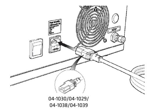
Select the appropriate **mains cable** from the fittings kit and plug the **IEC 60320/C19** cable into the **mains input** at the side of the generator.
