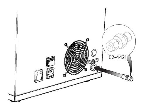
Attach the 1/4" Compression Fitting 02-4421 to the generators gas outlet.
