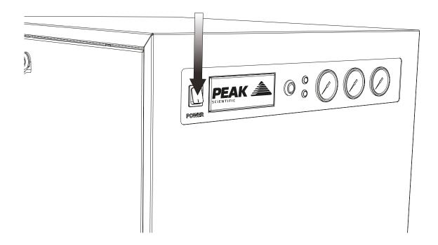
Again, Switch the generator power **ON** using the switch on the front panel.
