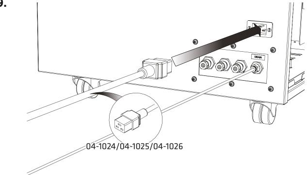
Select the appropriate **IEC 60320/C19** mains cable from the fittings kit and plug the cable into the mains input at the rear of the generator.
