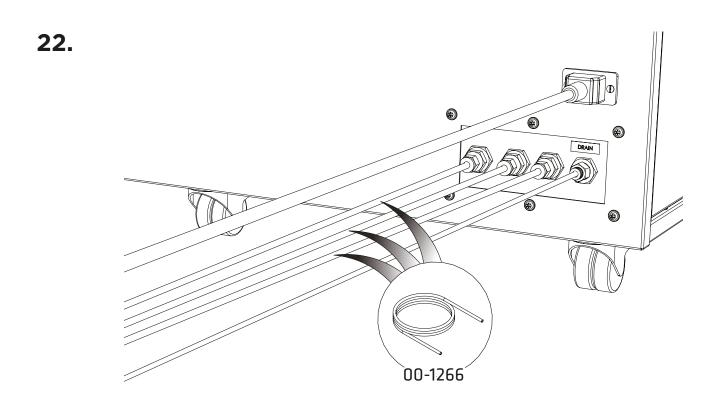
Attach the 1/4" **Teflon tubing 00-1266** to the fittings attached to the **CURTAIN**, **SOURCE & EXHAUST** and connect to the corresponding **gas inlets of your instrument**.
