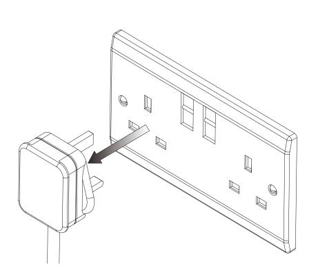
Remove the mains cable completely from the power supply.
