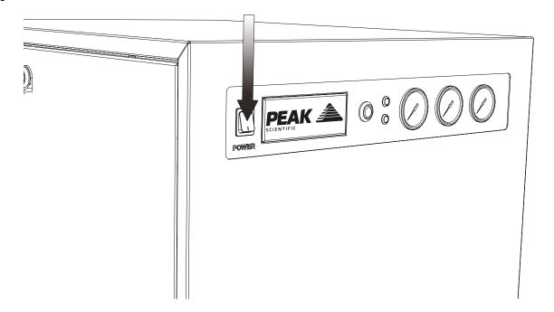
**After 30 minutes** of running, the generator can be turned **OFF**. Allow the stored gas in the internal tanks to dissipate.
