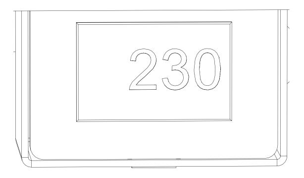
Check the Generators **internal voltmeter**. This will measure and display the mains voltage that is being supplied to the generator. Note the displayed voltage. If the voltage is 219V or less, we would highly recommend fitting a transformer. This can be ordered directly from Peak. **06-3200 Dual Tap Transformer 200-230V**
