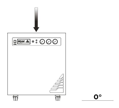
Unpack the generator from the shipping crate and position on a flat surface, in desired area.
