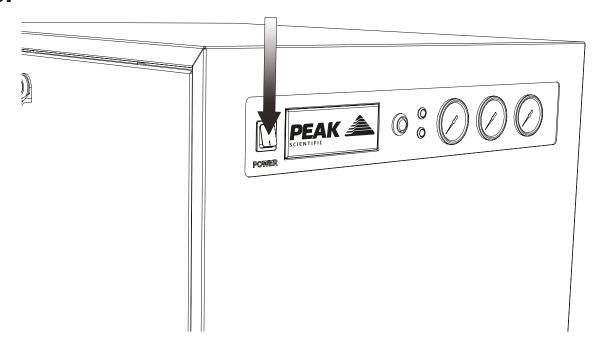
Switch the generator power **ON** using the switch on the front panel.
