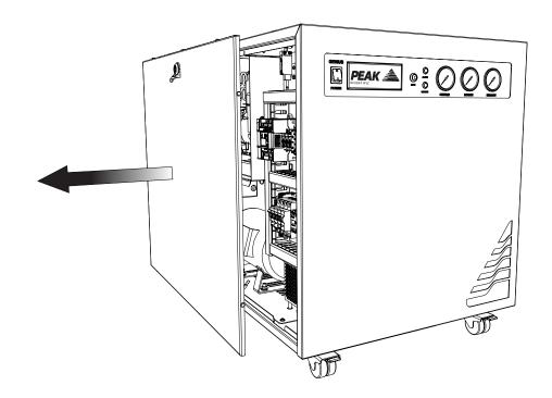
Once unlocked **remove the left hand side panel**, ensuring you **disconnect the earth lead** located in the lower middle of the panel.
