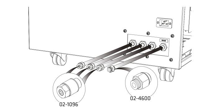
Select the 1/4"- 6mm Push Fit Fitting 02-4600 and attach to the Drain port at the rear of the generator.
