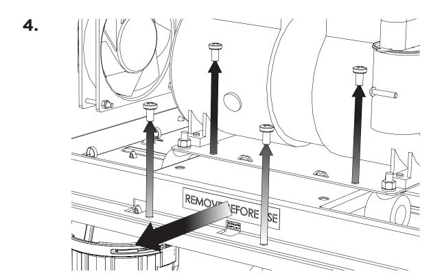
The **transit bracket** is located below the compressor and has a sticker on it stating 'Remove before use'. To remove the transit bracket, **remove the four screws** as indicated, then **slide the bracket out** from underneath the compressor. Please retain the bracket and screws for future transportation.
