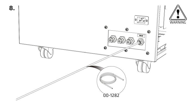
Connect the 6mm PE Tubing 00-1282 to the 1/4"- 6mm Push Fit Fitting 02-4600.
