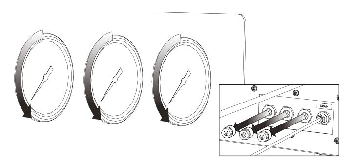
The purge is now complete. Once the pressure gauges on the front of the generator read 0, the **silencer fittings can be removed** from the Curtain, Source & Exhaust ports.
