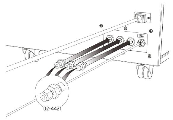
Select the 1/4" Compression Fittings 02-4421 and connect to the CURTAIN, SOURCE & EXHAUST ports.
