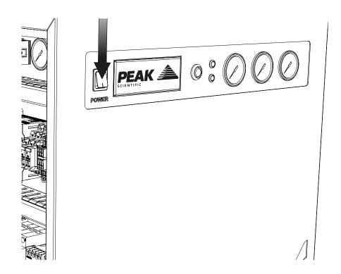
Switch the generator power **ON** using the switch on the front panel.
